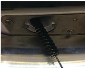
8. Use brush to clean nozzle connection ports on machine. BUNN Part No. 49827.0000.
