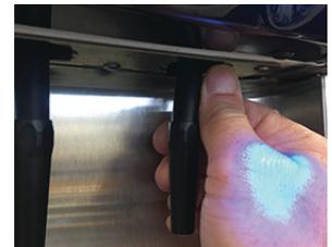
11. Replace drip tray and dispense nozzles. Be sure to install nitro nozzle in left dispense station.
