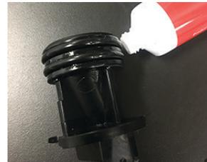
9. Apply small amount of food grade lubricant to o-ring on nozzles. BUNN Part No. M2550.0001.
