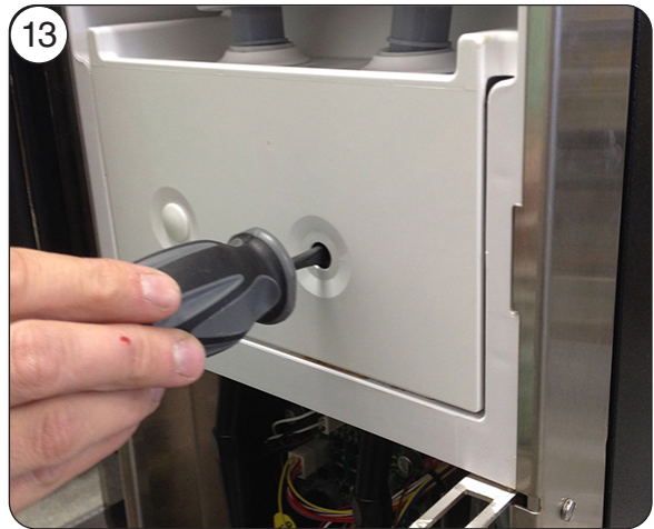
Adjusting Water Flow Using Flat Blade Screwdriver
