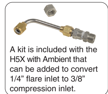
Plumbing Hook-Up for H5X with Ambient Side Dispense Only
