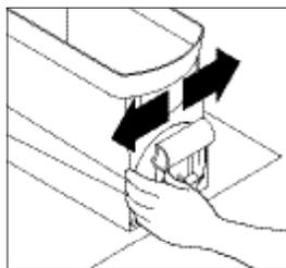
13. **CAUTION:** Faucet Valve is under spring tension. Spread one side of the Handle first, then the other and disconnect from the Hopper.
