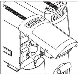
1. Open the Cabinet Door and allow the support arms to lock in place.
