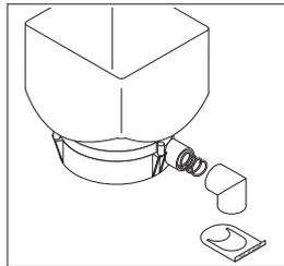
3. Pull the Ejector Elbow off the Hopper Base. Remove the Slide Gate from the Ejector Elbow.
