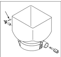
6. Remove the Auger Drive Shaft by removing Retaining Clip from Auger Drive Shaft.
