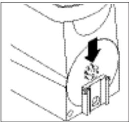
21. Replace the Auger Nose Bushing inside the front of the Hopper.
