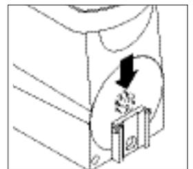
15. Remove the Auger Nose Bushing from inside the front of the Hopper.
