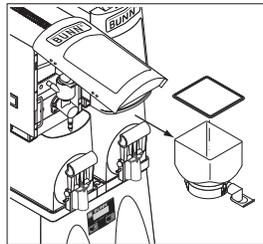
2. Remove the Hopper/Base Assembly from the Cabinet. Remove the Cover and empty the contents.
