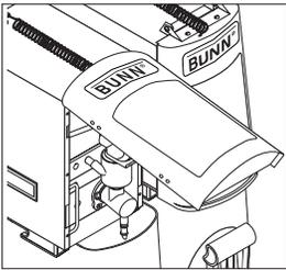
1. Open the Cabinet Door and allow the support arms to lock in place. Door must remain open during the entire cleaning procedure.
