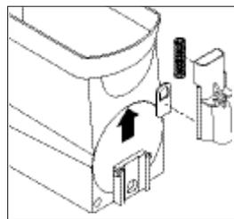
14. Carefully slide Valve up to remove Spring and Faucet Seal. Extra care should be taken when handling the Seal to prevent damage.
