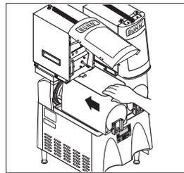
24. Install the Hopper over the Auger and Cooling Drum and slide it into place.
