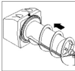
23. Align the Auger Shafts with the Augers. Push the Augers as far as they will go and rotate them so the flat face of the Auger Shaft is aligned with the flat face of the Auger nose.
