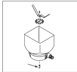
4. Remove the Wiper Blade and Drive Gear by removing the Retaining Ring from the Wiper Blade Shaft.
