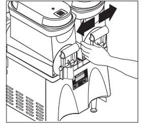
30. Press down on the Valve to compress the Spring. Position the Faucet Handle over the Faucet Valve one side at a time and snap into place on the Hopper.
