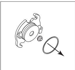
6. Slip the O-ring off the Whipper Chamber Receptacle and remove the shaft seal.
