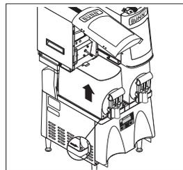
9. Depress the Hopper Lock Plunger, lift slightly.
