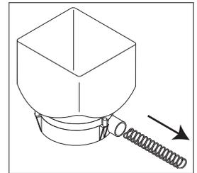
5. Remove Auger by pulling it out the front of Hopper Base.
