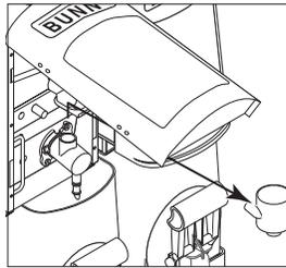
2. Pull the Mixing Chamber out of the Whipper Chamber.
