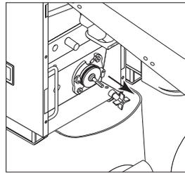
4. Pull the Frother off the Motor Shaft. Notice the flat keyway on the shaft and the matching keyway inside the Frother. It is important that these two keyways are lined up when reassembling.
