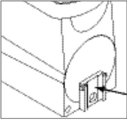
16. Do not scratch this surface when cleaning. Deep scratches could cause leakage around the seal.
