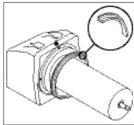
22. Install the Hopper Seal over the flange at the rear of the Cooling Drum as shown. Install Auger Shaft Seal (if used on this machine).
