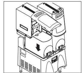
25. Push down until the Hopper Lock Plunger snaps into place.
