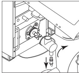
3. Twist the Whipper Chamber clockwise and pull it off the Whipper Chamber Receptacle.
