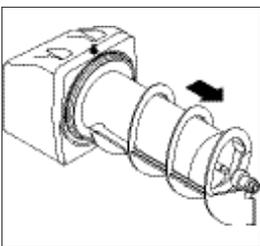
11. Pull the Auger from the Cooling Drum.
