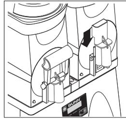
29. Slide the Faucet Valve assembly into place on the Hopper.
