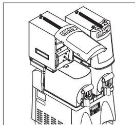
8. Slide PAF assembly back until it latches before removing ULTRA Hoppers.
