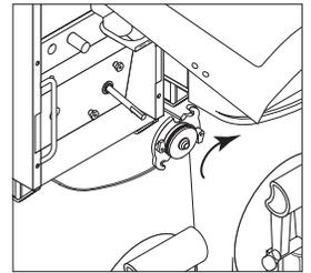
5. Twist Whipper Chamber Receptacle clockwise and pull it off the Motor Shaft.
