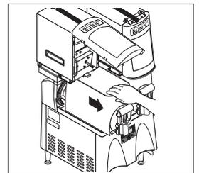
10. Pull the Hopper assembly forward and remove.
