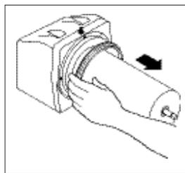
12. Remove the Hopper Seal from the flange on the Cooling Drum. Remove Auger Shaft Seal (if used on this machine).
