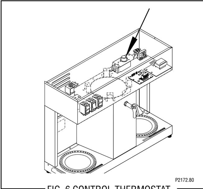
FIG. 6 CONTROL THERMOSTAT
